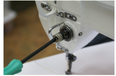
Fig 27: For fine adjustment of check spring insert screwdriver turn clockwise for more tension
