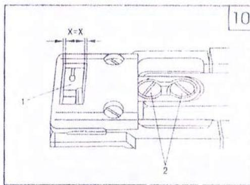
2. Positioning the feed dog in the direction of sewing (Fig.11)
