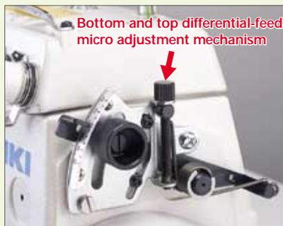
Bottom and top differential-feed micro adjustment mechanism
