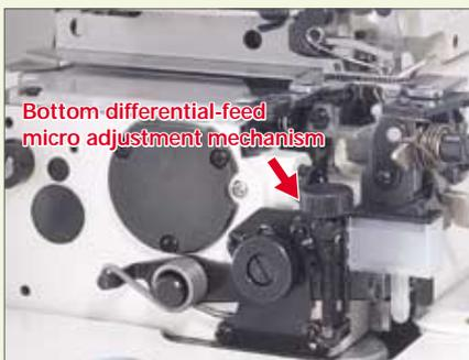
Bottom differential-feed micro adjustment mechanism
