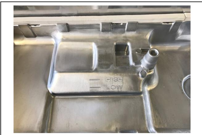
1. Be sure to supply oil when the oil level drops below the LOW baseline of the oil pan.
